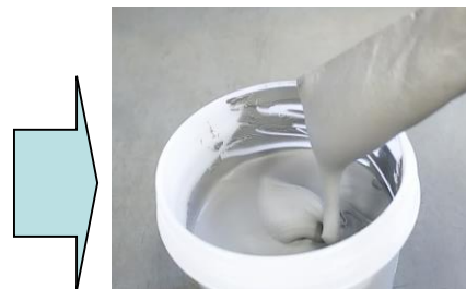
7日間継ぎ足し印刷後のソルダークリームの状態 (良好) The solder cream condition after printing for 7 days (excellent)
